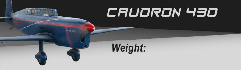
Max Weight: 820kg Empty Weight: 480kg Main Fuel Tank: 250kg Secondary Fuel Tank: NA///
